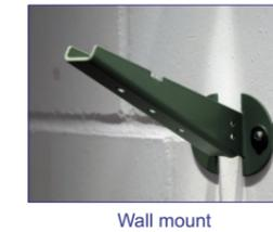
The profile should be installed at a vertical distance of approx. 15% of the height of the advertising space to be illuminated or at least 10 cm above or below the advertising space. The maximum permitted spacing between the wall mounts is 1 m.
