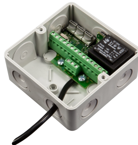
The DMX interface with the housing lid removed
